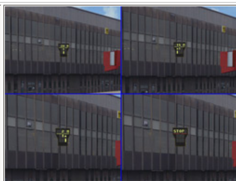
The AGNIS in action. The system counts down in increments of 5m from 30m, until you get to 5m, where it counts down in sets of 1m.
