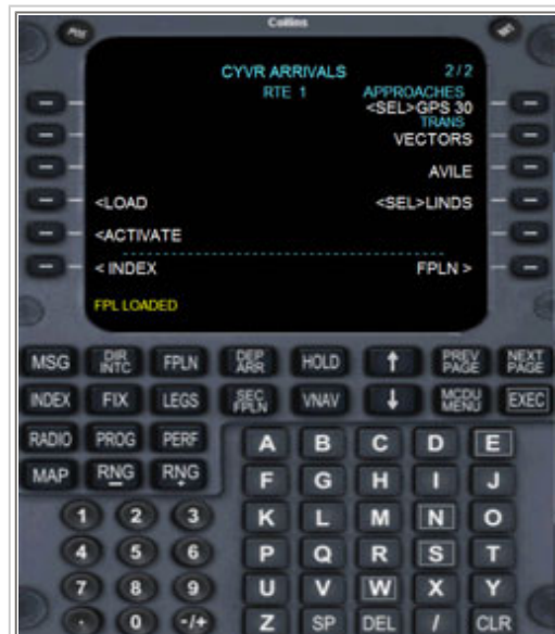
The DEP/ARR page can be used to find standard approaches and departures.
