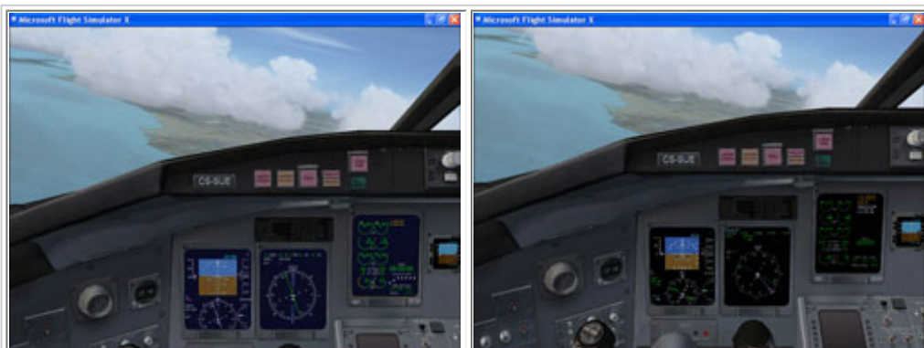
FSX and Friendly Panels daytime 3D Cockpits side-by-side: FSX on the left, Friendly Panels on the right. The only differences are in the MFD displays.
