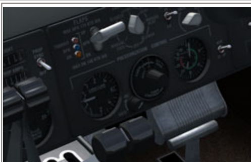
The environmental controls on the B60, one of many pre-zoomed sub panels available in the virtual cockpit
