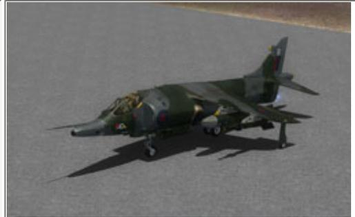
*233 Operational Conversion Unit GR3, fuel tanks and PaveLow loaded to hard points*
