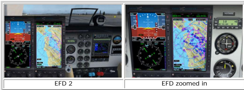
Compared to the standard steam gauges, the EFD panel gives you a wealth of information, complete with moving map. The panel also has a GPS (Garmin or KLN) installed, so you can program and follow GPS flight plans. I added my trusty Reality XP GNS530W and was happy to see that the avionics also support fully linked LPV approaches for the ultimate in flexibility.
