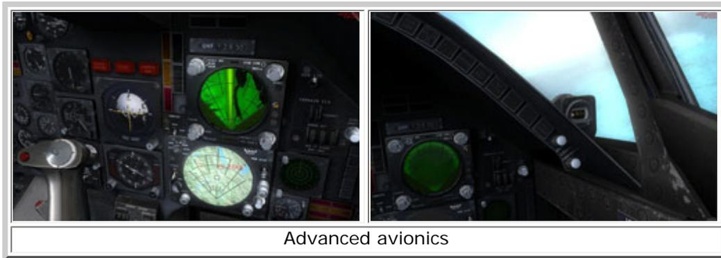
On the plus side -- and it's a much longer list -- Razbam has modeled the A-7's navigational systems in considerable depth. An attitude direction indicator (ADI) combines information that would normally be spread across two or three separate instruments: an artificial horizon, an OBS, and a gyroscopic compass. There's also a souped-up horizontal situation indicator (HSI) which, in addition to the usual VOR data, also displays bearing and distance info from NDB sources and the tactical computer.
