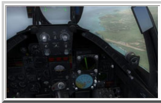
There's a three-axis autopilot, which can be used to hold heading and altitude. As is mentioned on the product web page, the real A-7 was equipped with an early version of autoland and autothrottle; what's not mentioned (and ought to be, in fairness to customers) is that Razbam's model does not implement either system. You can receive ILS signals, but not from any of the carriers (which you can do with the VRS Super Hornet or Jivko Rusev's freeware HUD for the Acceleration F/A-18).
