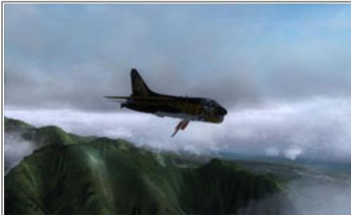
Speed brake deploys under the fuselage
